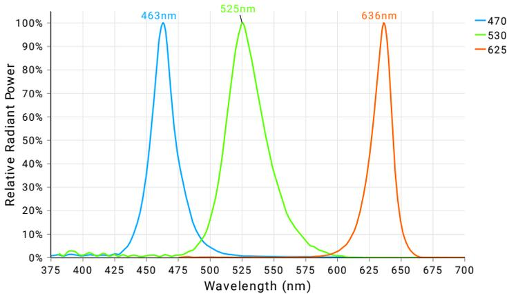
Visible color illumination consists of using wavelengths between 400-700 nm to either create or eliminate contrast on an inspection subject based on differences in a materials color hue. When referring to a color wheel, simply remember the following: like colors reflect and brighten surfaces; conversely, opposing colors absorb and darken surfaces.
