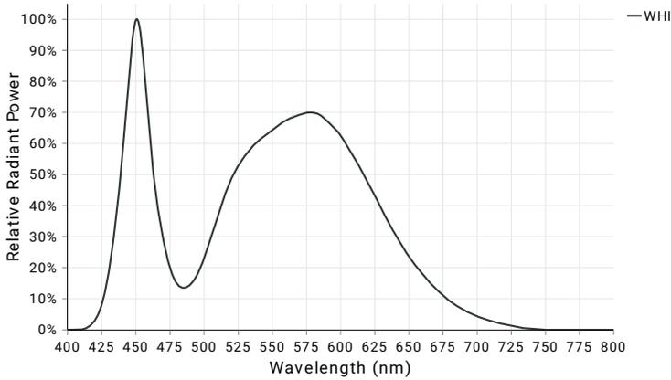
White LED illumination is the most commonly used machine vision lighting configuration. It is often the default choice when specific features of interest do not require color-based highlighting. However, white LEDs can vary in color temperature between different lighting families, which can impact machine vision systems, specifically when matching white light sources.
