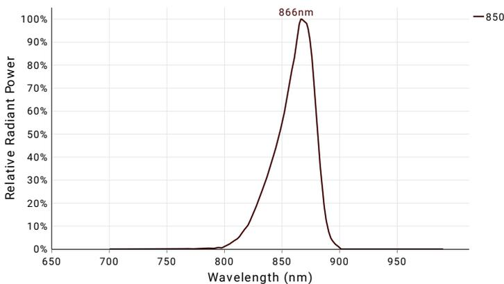
Near-infrared (NIR) imaging is a machine vision technique using longer wavelengths of 700-1000 nm to penetrate specific materials that are otherwise opaque under the visible spectrum. When paired with a NIR camera, a NIR light can be ideal for applications such as fill level inspection, circuit board inspection, food safety inspection, and medical imaging.
