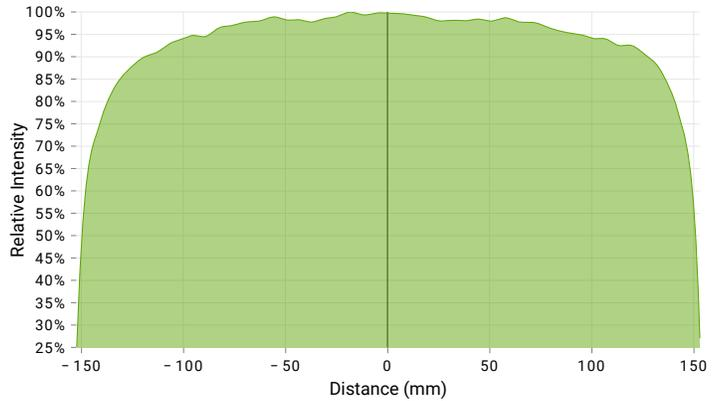
The BL2 Series provides a highly uniform output across its emitting window with an edge effect of only 17.3 mm, and a uniformity of +/- 10% within the optical area.
