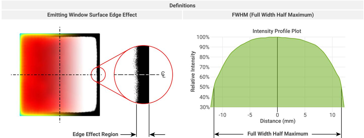
Edge Effect refers to the decrease in light intensity along the outer perimeter of a backlight's emitting surface. It's characterized by the region where the intensity falls below 80% of the peak value. For linear backlights, edge effect is measured along the length of the light. We recommend users avoid this region when sizing a backlight for their application.
