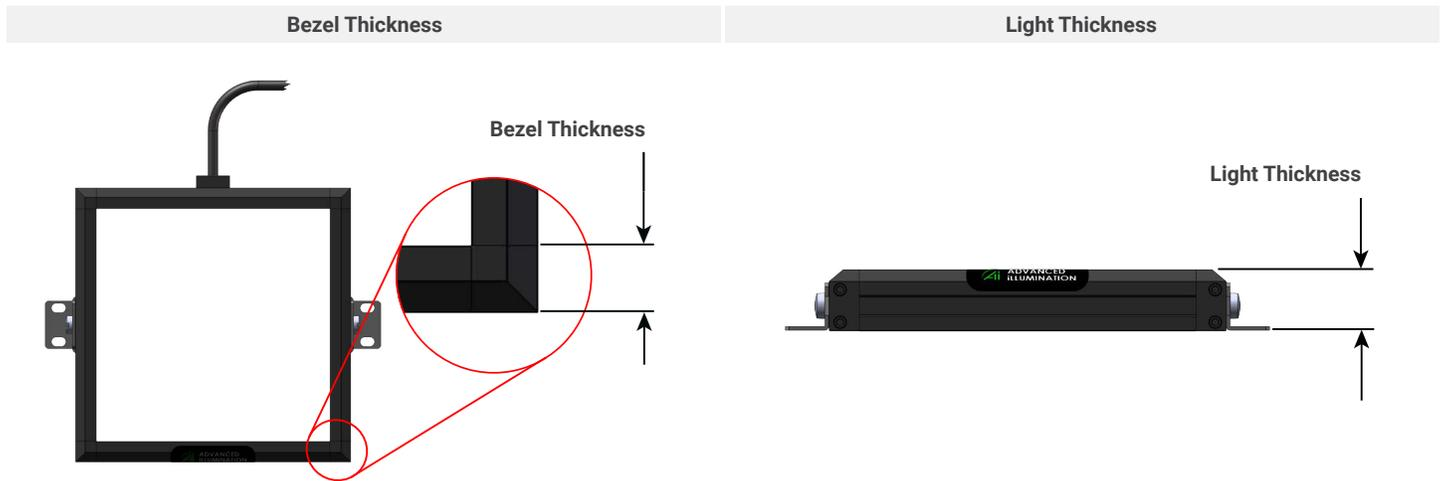
Bezel Thickness refers to the width of the non-illuminated border or frame surrounding the light-emitting surface of a machine vision backlight. Bezel thickness is an important consideration when integrating a backlight into a tight space, as it directly affects how close you can place the light-emitting surface to an object on its side.
