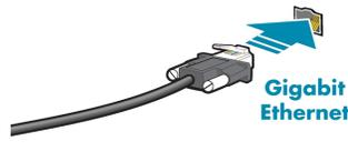
Plug the interface cable into the host controller card and the camera. The cable jack screws can be used for a secure connection.
