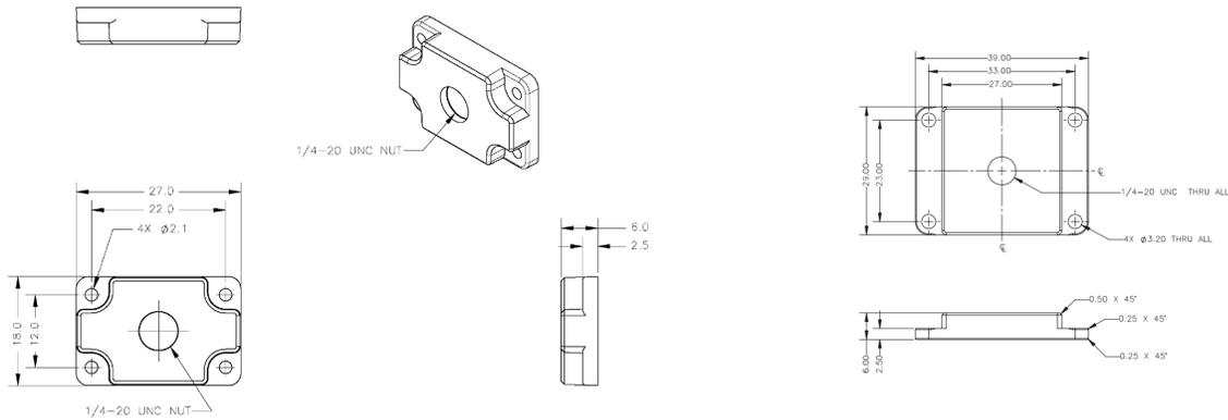
**Tripod Adapter Dimensional Diagram
