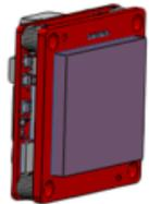
The sensor is covered with a protective sticker. Remove the sticker. If any residue is present, clean the sensor surface with a non-abrasive cotton swab and isopropyl alcohol cleaning solution. Immediately install the image board over the prepared lens mount.
