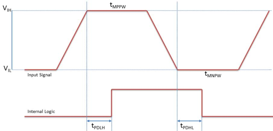
**Opto-isolated Input Performance ( $V_{cc}$  = varying pk-pk)**
