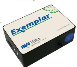
The Exemplar® was the first smart spectrometer to feature on-board data processing, USB 3.0 communication, and temperature compensation. The Exemplar is also optimized for multi-channel operation featuring ultralow trigger delay and gate jitter. Additionally, the Exemplar features a 2048 element detector and built-in 16-bit digitizer with greater than 2.0 MHz readout speed.
