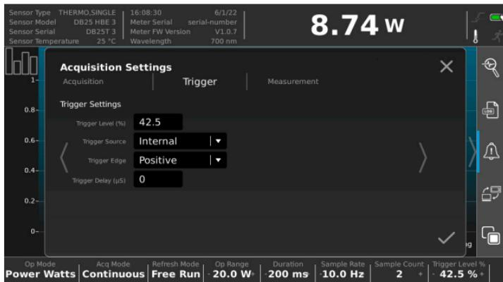
**Figure 17. Acquisition Settings - Trigger**
