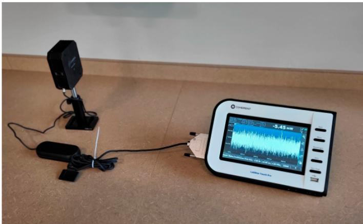
**Figure 9. Connect the Meter to a Sensor**
