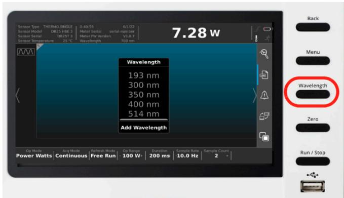
**Figure 16. WAVELENGTH and ZERO Function Buttons**
