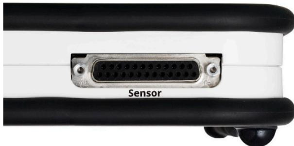
**Figure 2. 25-pin connector**
