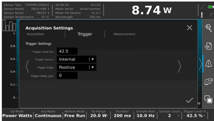
**Figure 21. Acquisition Settings - Trigger**
