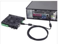
Stand-alone controllers also have the option to connect directly to a computer's USB port with a U-DC06† cable.
