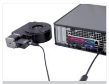
X-Series devices can connect to a computer's USB port with an X-USBDC\* cable.
