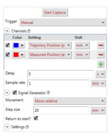
Press Start Capture to begin reading the information. The device will move, and once all of the data has been collected and transmitted, a plot of the information will be displayed.
