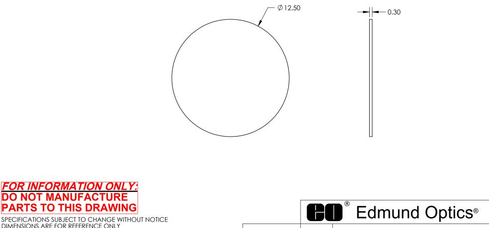
DIMENSIONS ARE FOR REFERENCE ONLY Everix Ultra-Thin OD 4 Notch Filter, 642nm, THIRD ANGLE S2 TITLE S1 12.5mm Diameter PLANO PLANO SHAPE SHEET ALL DIMS IN DWG NO mm Ø11.25 Ø11.25 23680 CLEAR APERTURE 9 OF 15
