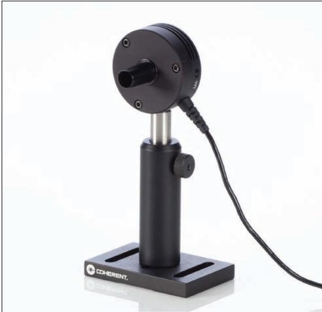
The Quantum EnergyMax sensor incorporates a Silicon photodiode, contains a large 10 mm clear aperture and operates at a repetition rate from single pulse up to 10 kHz (every pulse).
