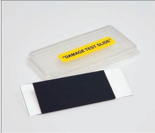
For protection of your sensor when measuring unknown beams, the test slide is inserted into the beam and then examined for damage. These test slides are coated with the same absorbing coating as the pyroelectric sensors. If coating damage is visible, then attenuation is required before measuring the beam.
