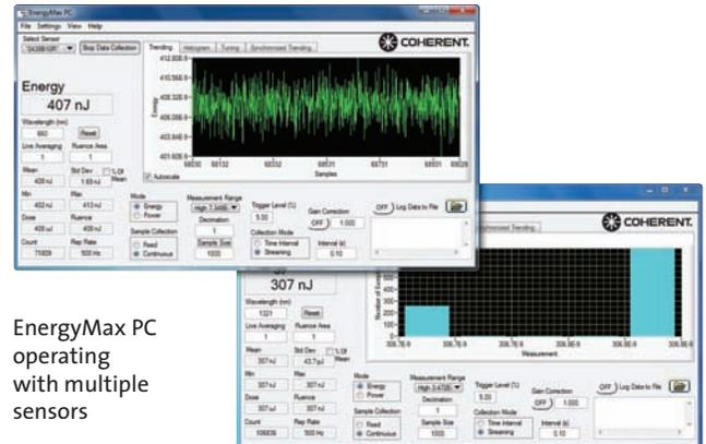
EnergyMax PC operating with multiple sensors
