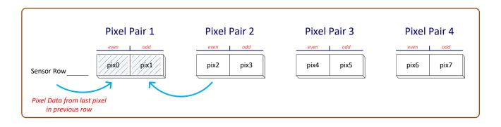
When a row's last pixel pair has both even and odd pixels marked as bad, the even pixel is
