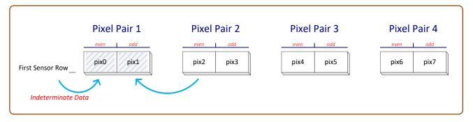
• When the first pixel pair of an image row has both even and odd pixels marked as bad, the even pixel is replaced by pixel from the preceding row's last pixel. The bad odd pixel is replaced by the following even pixel (even if it is also marked as a bad pixel).
