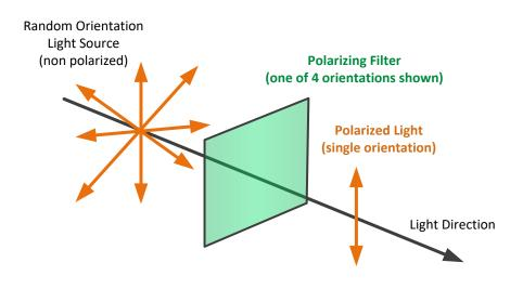
The Genie Nano's polarizer filter on the camera sensor is implemented as a 2x2 pattern, with each pixel having a nanowire polarizer filter with a different angle (90°, 45°, 135°, 0°).
