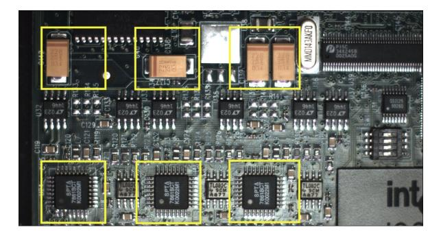
With the ROI areas defined, the camera outputs an image consisting only of data within those ROI areas, as shown below. Such data reduction improves transfer bandwidth and also reduces image processing time for the host system imaging application.
