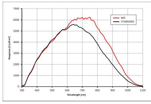
On-Semi Python Series (16M & 25M with 4.5  $\mu m$  pixels) — Monochrome and NIR
