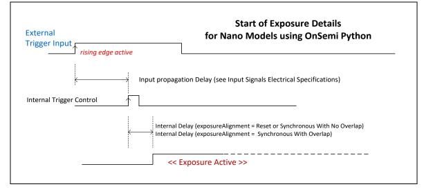
Additional triggered exposure mode features and timing specific to OnSemi sensors are described in the <u>I/O Controls Category</u>.
