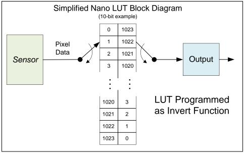
Simplified Example 10-bit LUT Block Diagram
