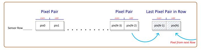
When the sensor's last row's last pixel pair has both even and odd pixels marked as bad, the even pixel is replaced by preceding odd pixel and the bad odd pixel is replaced by indeterminate data in the following memory location.
