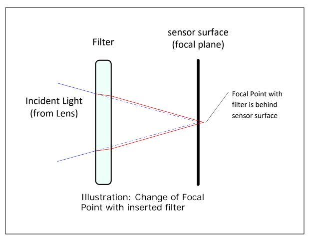
In this example when a glass filter is inserted between the lens and the camera sensor, the focal point is now about 1/3 of the filter thickness behind the sensor plane. Genie Nano filters are specified as 1mm thick.
