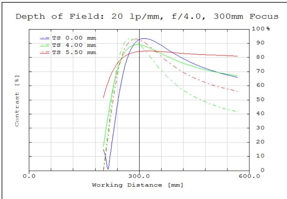
**Figure 4:** Polychromatic diffraction through-focus MTF at 20 linepairs/mm (image space). Contrast is plotted to two times the focus distance. Note object spatial frequency changes with working distance.
