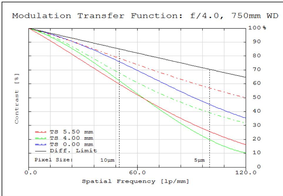
**Figure 5:** Image space polychromatic diffraction FFT Modulation Transfer Function (MTF) for  $\lambda = 486\text{nm}$  to  $656\text{nm}$ . Included are the Tangential and Sagittal values for field points on center, at 70% of full field and the maximum sensor format. Solid black line indicates diffraction limit determined by  $f/\#$ -defined aperture. Frequencies corresponding to the Nyquist resolution limit of pixel sizes are indicated.
