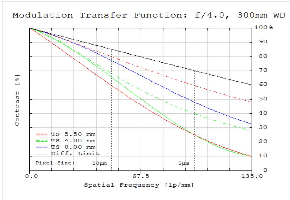
**Figure 3:** Image space polychromatic diffraction FFT Modulation Transfer Function (MTF) for  $\lambda = 486\text{nm}$  to  $656\text{nm}$ . Included are the Tangential and Sagittal values for field points on center, at 70% of full field and the maximum sensor format. Solid black line indicates diffraction limit determined by f/#-defined aperture. Frequencies corresponding to the Nyquist resolution limit of pixel sizes are indicated.
