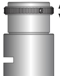
5. Thread entire assembly into C-Mount camera from the top of Rear Assembly until the top of the Locknut is flush against the camera C-Mount.
