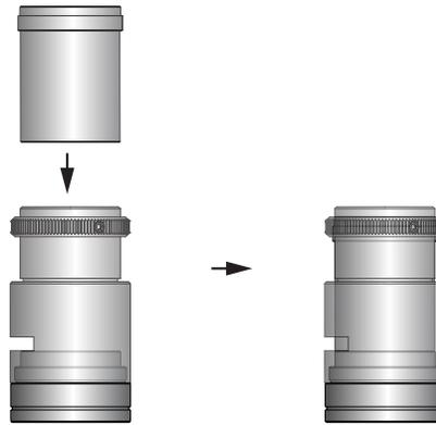
4. Adjust Locknut position until desired focus is achieved. See section on Working Distance and Field of View below to find Locknut positions. Tighten Nylon Tip Set Screw into place for a focal position that can later be readjusted—the nylon tip will protect the threads. To set focal position permanently, install the socket head screws. Do not overtighten screws.
