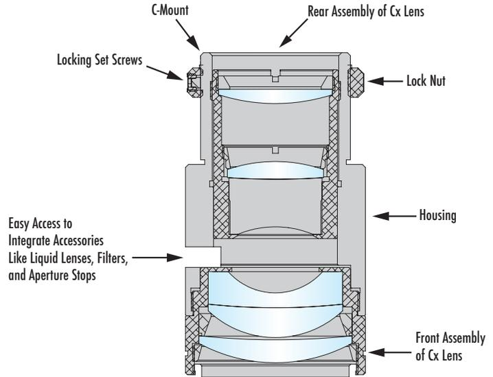
**Figure 1:** 50mm Cx lens without the required accessory.
