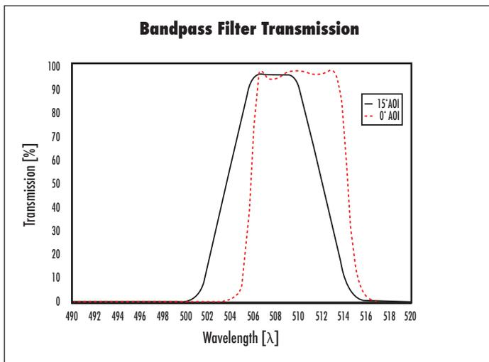
**Figure 3:** The graph to the left shows the effect of using a bandpass filter at a 15° angle of incidence compared to an incident angle of 0° (surface normal). The center wavelength shifts toward shorter wavelengths, and the overall transmission profile of the filter is compromised. The optical density of the filter also lowers, broadening the FWHM (Full Width Half Max).
