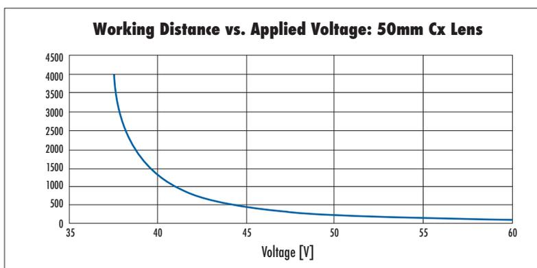
**Figure 5:** Working distance as a function of voltage applied to liquid lens for 50mm Cx Lens.
