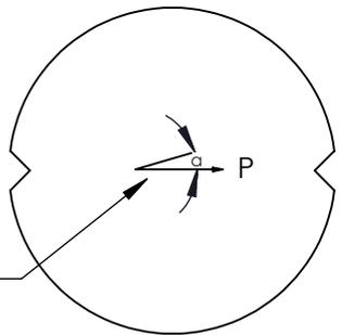
POLARIZATION AXIS P  $\alpha = 0^\circ \pm 2^\circ$
