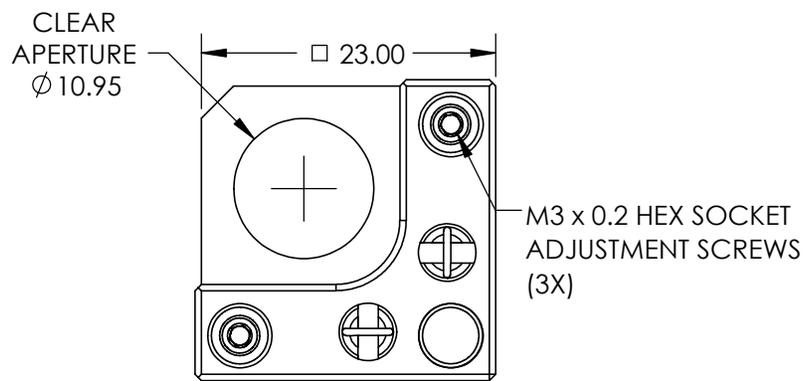
M3 ADJUSTMENT LOCKING HEX SOCKET SET SCREWS (3X)
