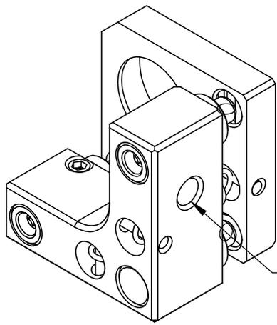
M4 x 0.7 x 7 DEEP FOR MOUNTING THE KINEMATIC ASSEMBLY (2X)
