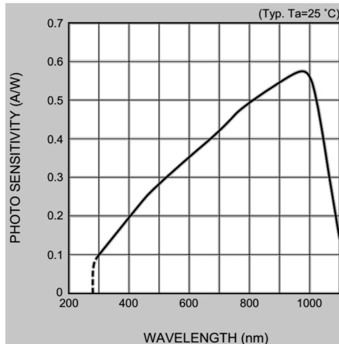
Fig 2. Typical Spectral Response for EO100-Si-HA-OD1
