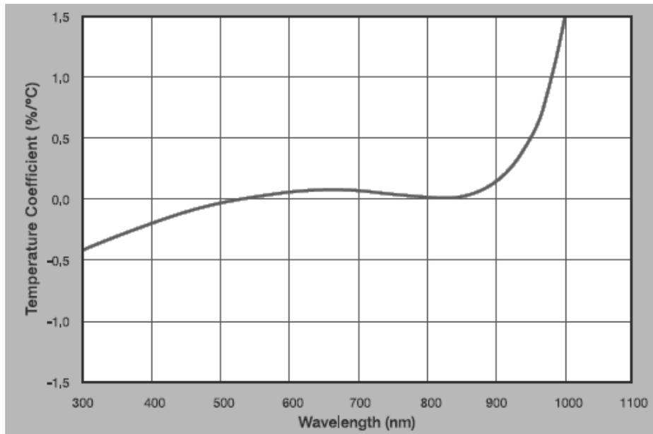
Fig 1. Typical Si and SiUV temperature dependence vs wavelength
