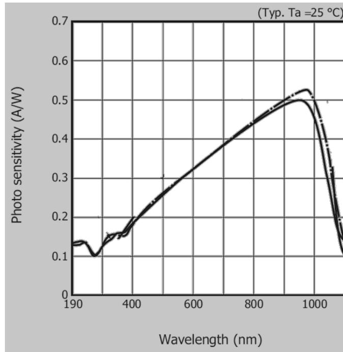
Fig 3. Typical Spectral Response for EO100-SiUV-OD.3
