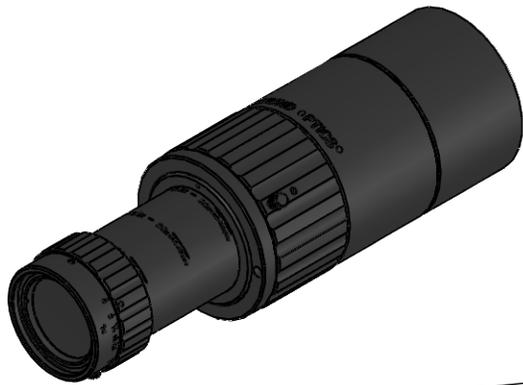
153.69mm OVERALL LENGTH @ MIN WORKING DISTANCE  $\triangle 2$
